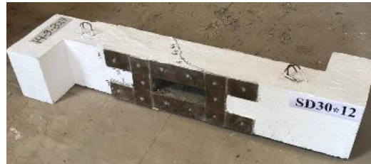
(b) Crack pattern for SD30x12
