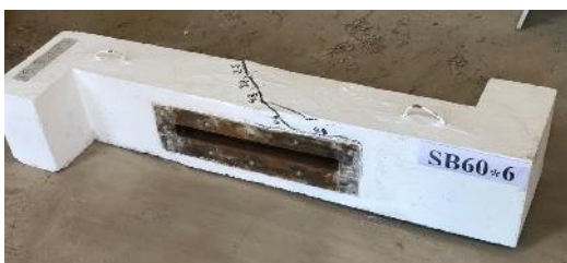
(c) Crack pattern for SB60x6
