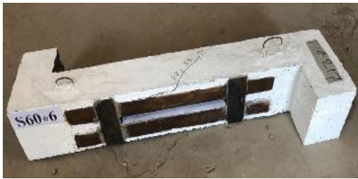
(c) Crack pattern for S60x6
