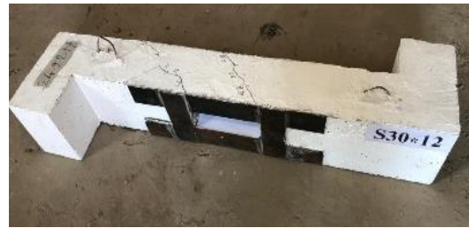
(b) Crack pattern for S30x12
