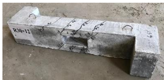
(c) Crack pattern for R30*12
