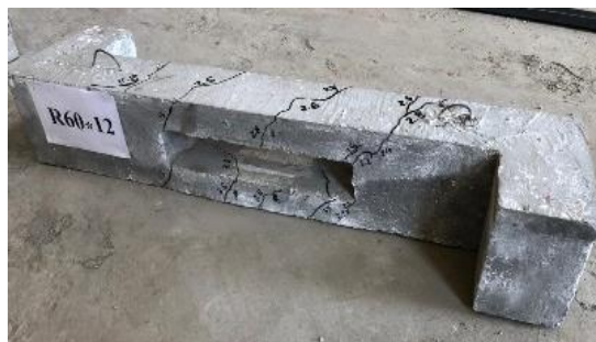
(e) Crack pattern for R60*12
