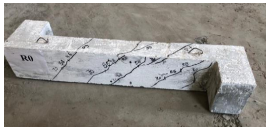
(a) Crack pattern for beam R0
