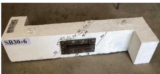
(a) Crack pattern for SB30x6
