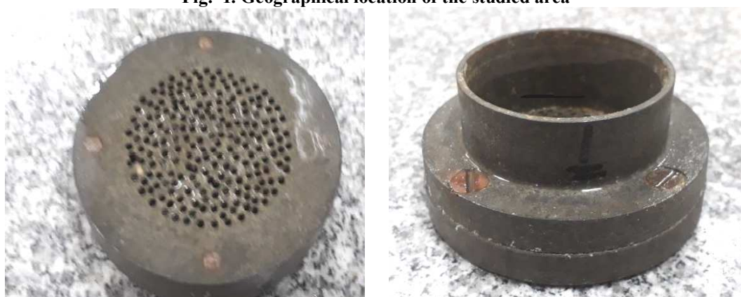
Fig. 2. A metal cylinder used for measure soil shrinkage
