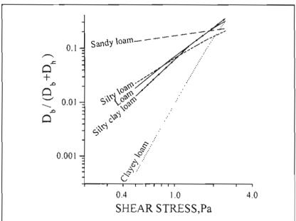
Figure 7. Predicted bed-scour detachment ( $D_b$ ) as a fraction of predicted total detachment (sum of bed scour and head cut,  $D_b + D_h$ ) using the power function ( $D = K \tau^b$ ) vs. shear stress for five soils.
