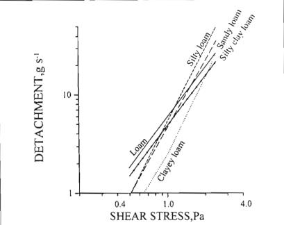
Figure 6. Predicted head-cut detachments using the power function  $(D = K\tau^b)$  vs. shear stress for five soils.
