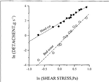
Figure 4. Detachments due to bed - scour and head - cut processes as a function of shear stress for natural log-natural log transformed data for a silty loam soil.
