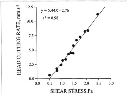
Figure 2. Head-cutting migration rate as a linear function of shear stress for a silty loam soil. Each point represents the mean of four replicates.
