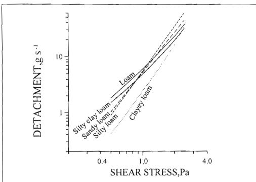
Figure 8. Predicted total detachment (sum of bed-scour and head-cut,  $D_{\mathfrak{b}}+D_{\mathfrak{h}}$ ) using the power function ( $D=K\mathfrak{T}^{\mathfrak{b}}$ ) vs. shear stress for five soils.
