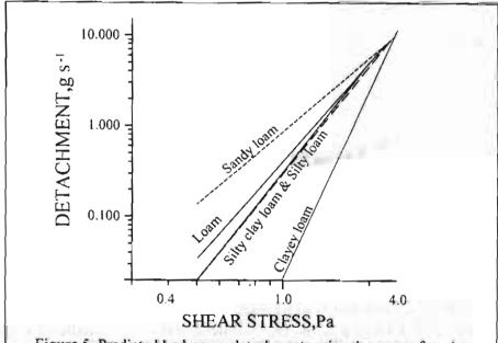
Figure 5. Predicted bed-scour detachments using the power function ( $D = KC^b$ ) vs. shear stress for five soils.
