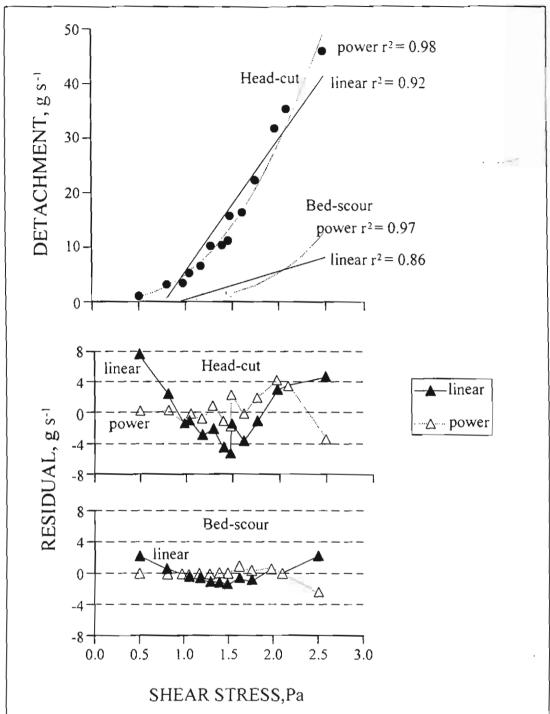
Figure 3. Bed-scour and head-cut detachments vs.shear stress for a silty loam soil and their respective residual deviations from predicted values using the linear {  $D = K(\tau - \tau_c)$  } and power (  $D = K\tau^b$ ) regressions.
