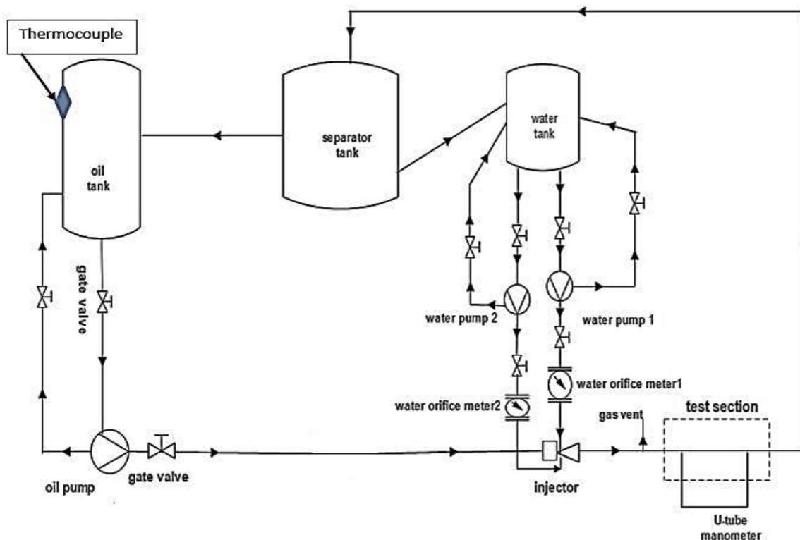
Fig. 2. Schematic diagram of the experimental test rig
