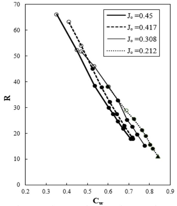
Fig. 18. Pressure drop reduction factor (R) as function of water input ratio ( $C_w$ ) for Case 2
