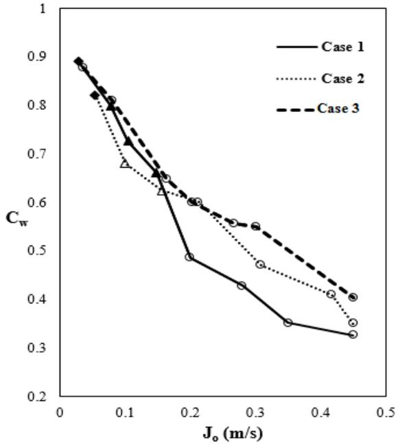
Fig. 20. Maximum water input ratio corresponding to  $R_{\max}$  as function of oil flow rate;  $\blacklozenge$ =dispersion oil in water;  $\blacksquare$ =plug;  $\blacktriangle$ =slug;  $\triangle$ =wavy stratified;  $\bullet$ =core-annular;  $\circ$ =wavy annular.
