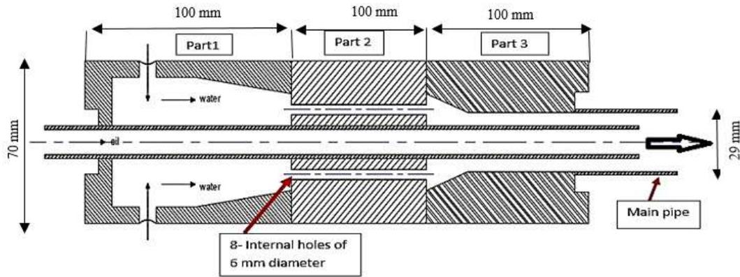
Fig. 3. Schematic diagram of the fluid injector
