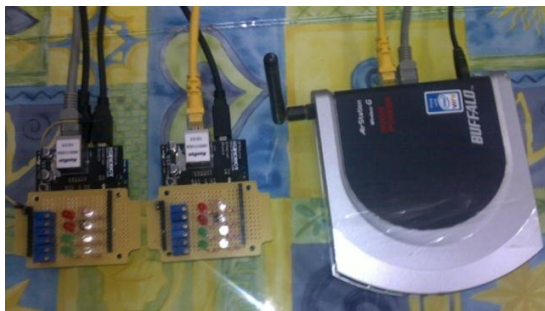
Figure 18 , Two RTU's with Air Station Wireless High Power Module.
