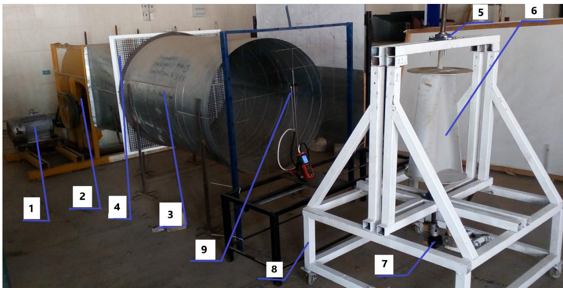
(1) AC motor (2) Centrifugal fan (3) Duct (4) Grid (5) Bearings (6) Rotor (7) Torque meter (8) Frame (9) Pitot tube
