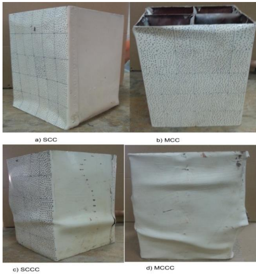
a) SCC b) MCC c) SCCC d) MCCC Fig.12. Experimental failure mode and deformation shape at failure
