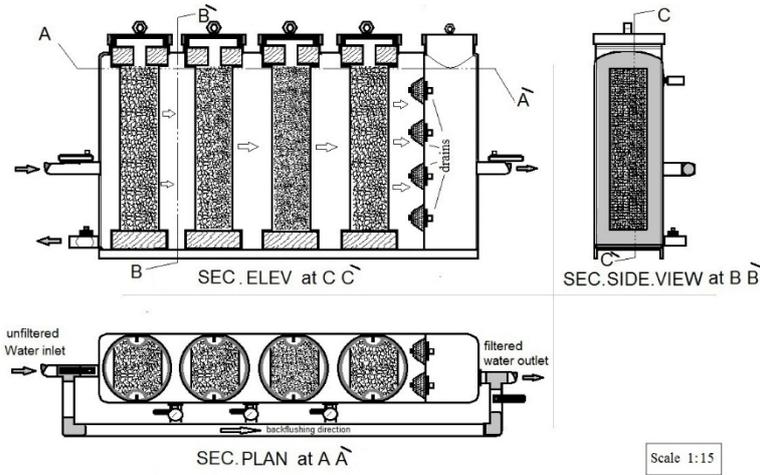
**Fig (3): Sectional views of elevation, side view and plan with the water movement across the proposed filter.**
