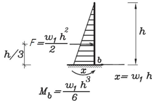
**Fig (1) Pressure distribution inside the filter column.**
