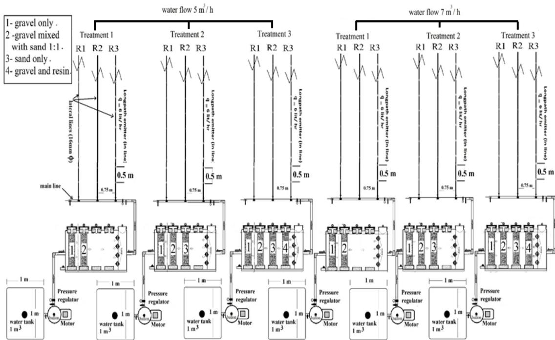
**Fig (6):** A schematic diagram of the tested treatments for both Nile and mixed agricultural drainage water under 5 and 7 m<sup>3</sup>.h<sup>-1</sup> of water flow rate inside the new filter (6 treatments for each type of water).
