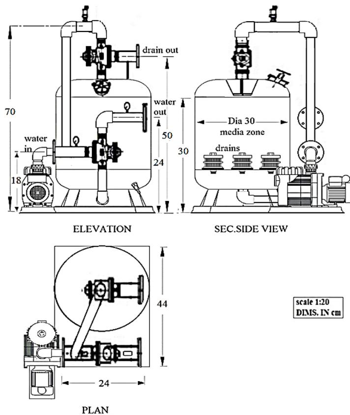
Fig (5): Elevation, plan and sectional side view of the used traditional sand filter with its components and dimensions.
