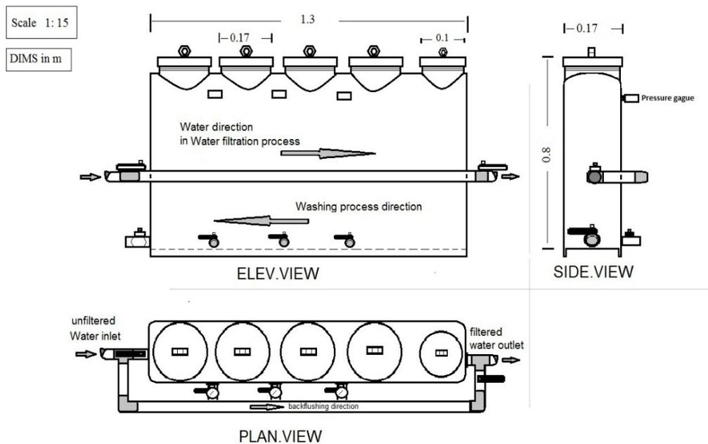
**Figure (2): The three views and dimensions of the proposed filter.**
