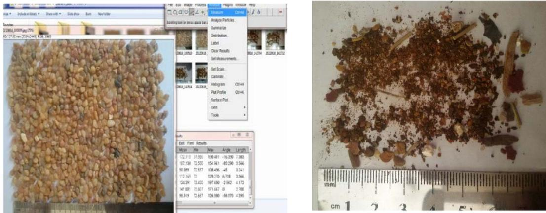
**Fig. (7):** Image Java Windows program used to measure grain media size and deposits before and after filtration process.
