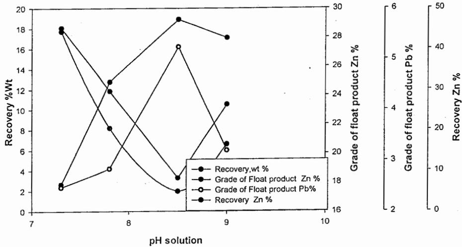
Figure (5) Effect of pH on the flotation tests of the selected sample
