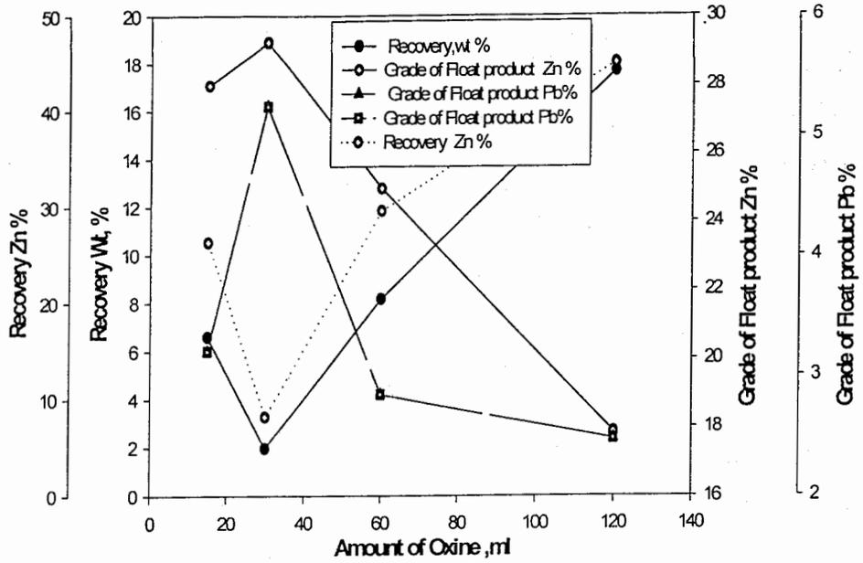
Figure (4) The effect of addition of the amount of oxine to float the zinc or
