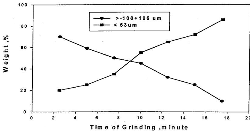
Figure(3) Weight % of ground products having >106 um and <53 um in diameter as a function of grinding time
