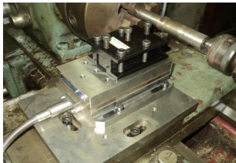
Fig. 1: Mounting of dynamometer on carriage of lathe.
