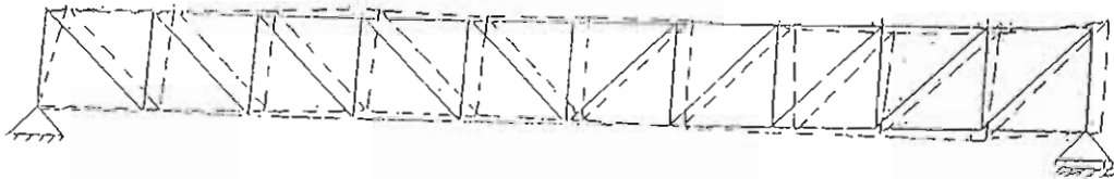
Fig (6-b) second mode shape with 1/m as uniformly distributed load (N-system truss)
