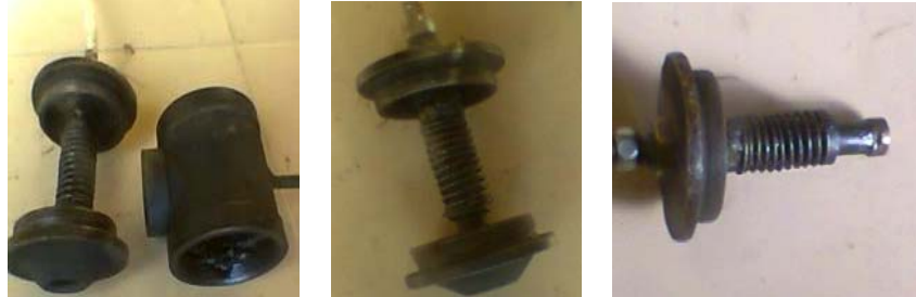
Figure 2: The ejector with a nozzle of 1.0 mm
