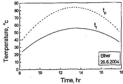
**Figure 3** Variation of working fluid and collector plate temperatures with time
