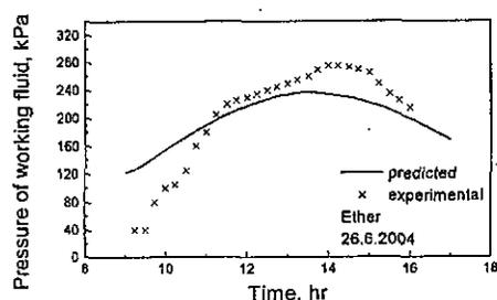
Figure 11 Calculated and measured working fluid pressure
