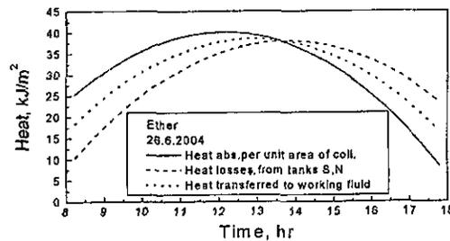
**Figure 4** Predicted values of heat absorbed per unit area of collector, heat losses from tanks S,N and heat transferred to working fluid
