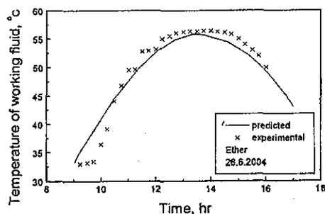
Figure 10 Calculated and measured working fluid temperature
