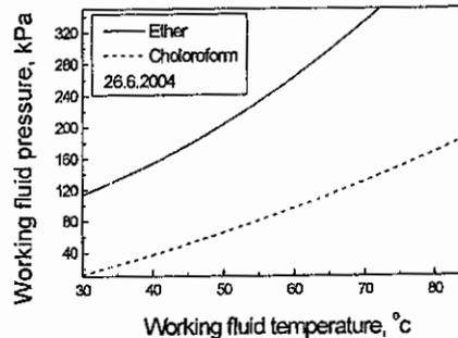
Figure 8 Variation of working fluid pressure with temperature
