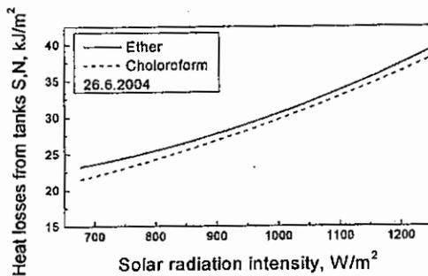
Figure 6 Effect of solar radiation intensity on heat losses from heat tanks S.N.
