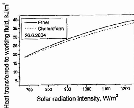
Figure 7 Effect of solar radiation intensity on heat transferred to working fluid
