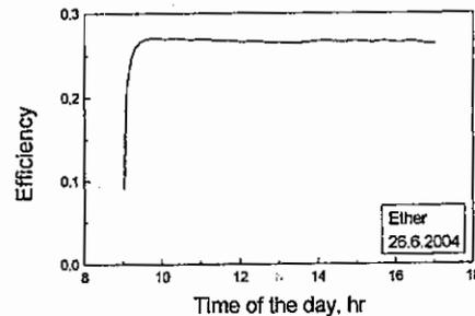
Figure 9 Variation of system efficiency with time of the day
