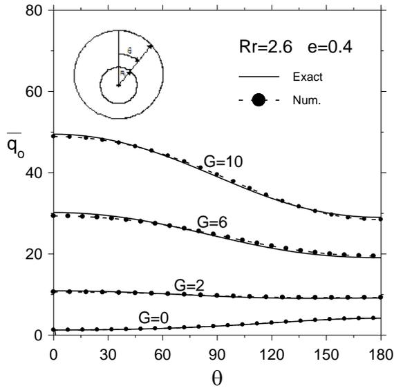
Figure 4- Heat flux along a) inner wall; b) outer wall at  $Rr=2.6$ ,  $e=0.4$  and at different values of  $G$ .
