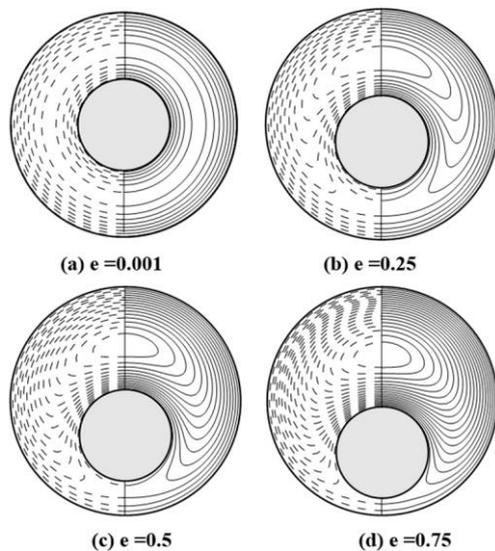
Figure 5- Patterns of exact isotherms (right) and numerical isotherms (left) for the case of eccentric enclosure at  $G=10$ ,  $Rr=2.5$  and a)  $e=0.001$  (almost concentric annulus), b)  $e=0.25$ , c)  $e=0.5$ , d)  $e=0.75$ .
