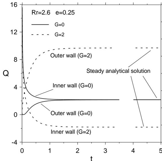
Figure 2- Time variation of numerical dimensionless heat transfer rates from inner and outer walls.
