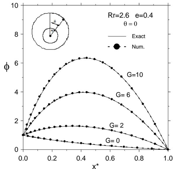
Figure 3- Distribution of dimensionless temperature in the gap along line of  $\theta = 0$  and at different values of  $G$ .
