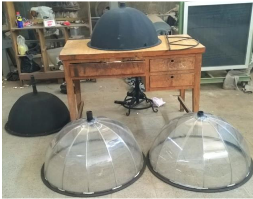
Fig. (2.1) Absorber and transparent cover of the collector
