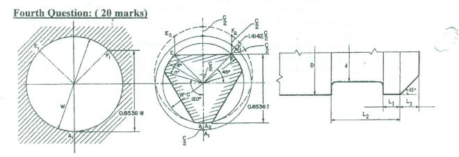
Figure shows a cylindrical locator with triangle relief. If the hole diameter"W" is  $82\pm0.005$  mm analytically calculate the dimensions of the required free jam locator (10 marks). Then graphically with suitable scale draw this locator (take the nearest integer number of your calculations in the locator's drawing) (10 marks). Given are,  $\mu = 0.3$ ,  $L_1 = 0.036$  D,  $L_2 = 0.8536\mu W$ ,  $L_3 = 1.55\sqrt{D}$ , and d = 0.95 D.
