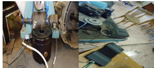
Fig.(1b) data acquisition system with vibration exciter for vibration testing
